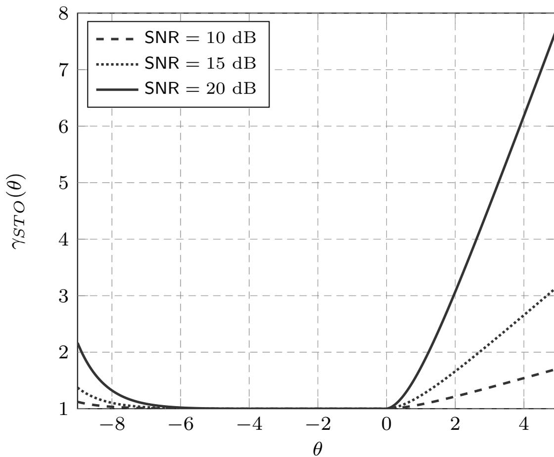
Figure 1.3: Performance decay due to STO -  $N = 128$ ,  $N_{CP} = 9$ , Exponential decaying channel with  $L = 8$
