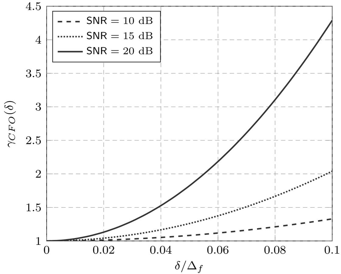
Figure 1.4: Performance decay due to CFO
