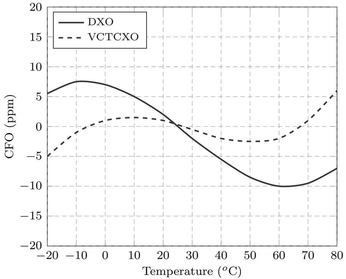
Figure 1.1: CFO effect on crystal oscillators due to temperature
