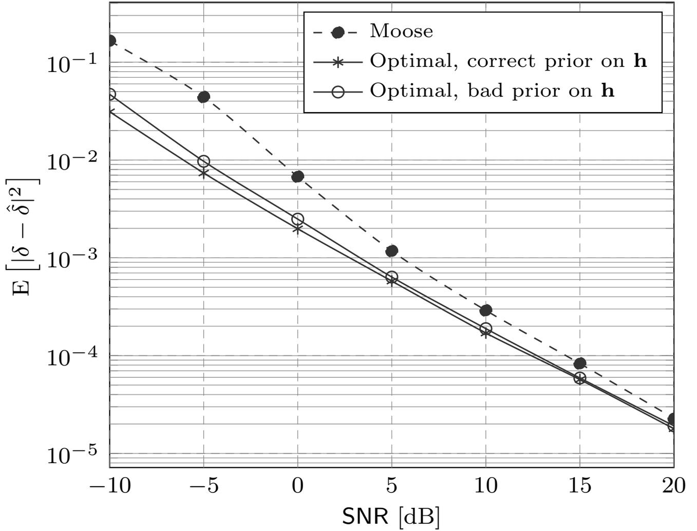
Figure 1.8: Optimal Bayesian CFO estimation - Comparison between Moose's methods [7] and Bayesian method. *Conditions:  $N = 128$ , random double-half OFDM symbol,  $\mathbf{h}$  is i.i.d. Gaussian with length  $L = 3$ , prior on  $\mathbf{h}$  either perfect:  $L_{as} = L$  or imperfect  $L_{as} = 9$*
