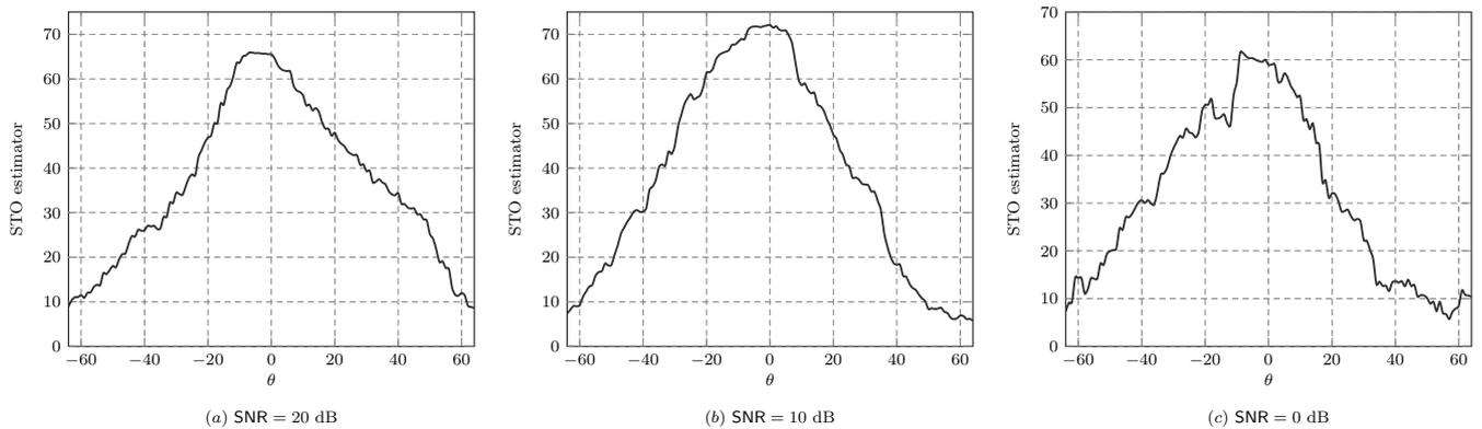
Figure 1.5: STO estimation for different SNR values,  $N = 128$ ,  $N_{CP} = 9$ , exponential decaying channel with  $L = 5$
