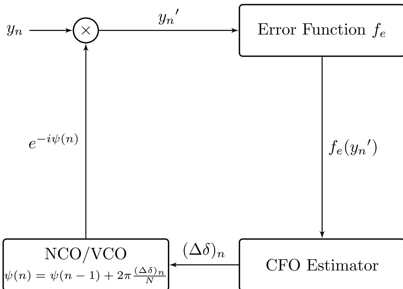
Figure 1.7: Closed-loop CFO tracking
