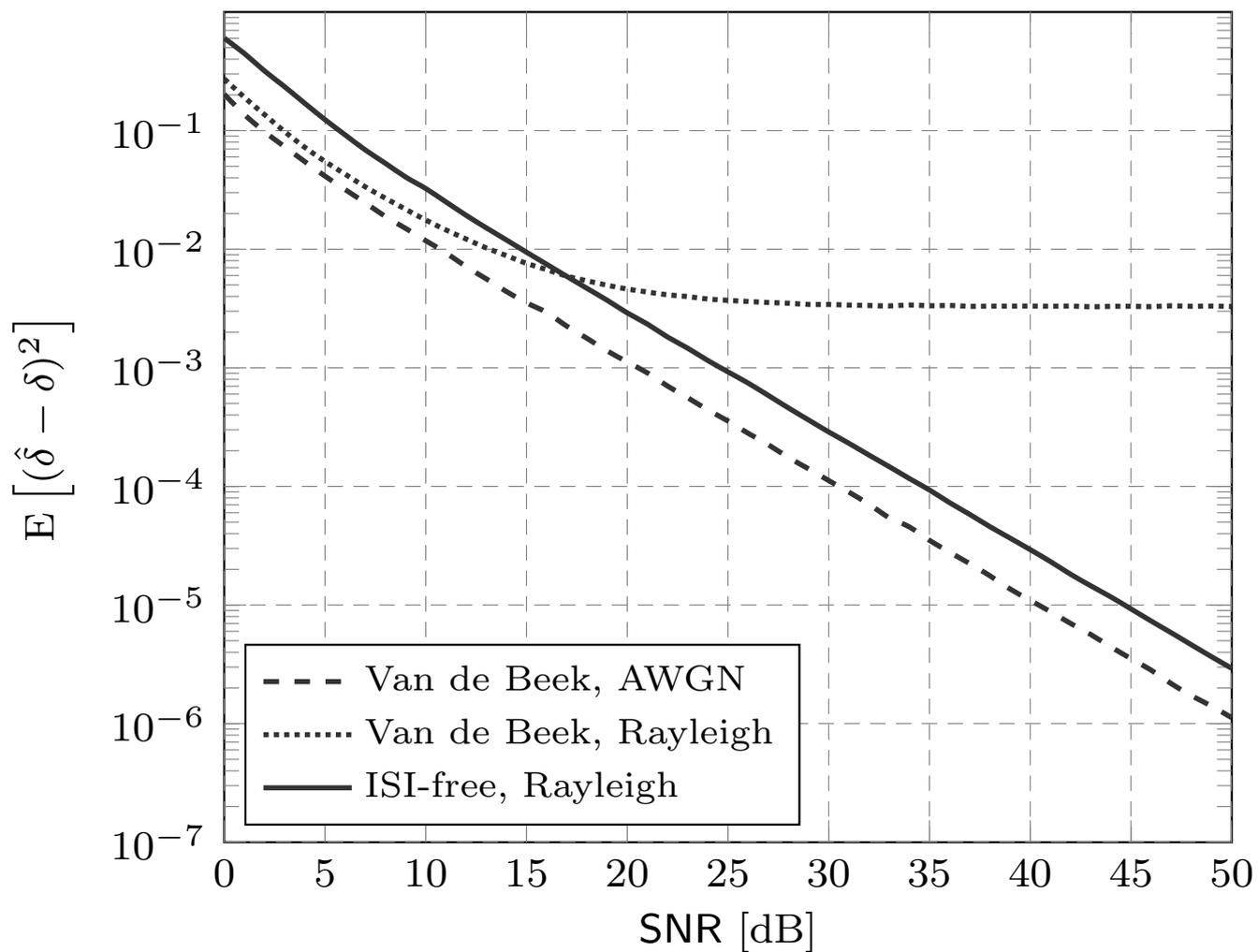
Figure 1.6: Rough CFO estimation versus SNR values,  $N = 128$ ,  $N_{\text{CP}} = 9$ , AWGN and Rayleigh channel with  $L = 5$
