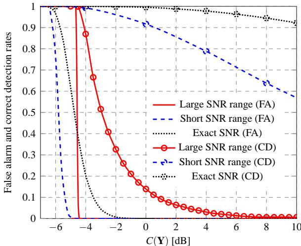
**Fig. 3.** False alarm (FA) and correct detection (CD) rates for exact, short discrete range ( $\{0, 2.5, 5\}$ ) and large discrete range ( $\{-5, -2.5, 0, 2.5, 5\}$ ) SNR -  $M = 1, N = 8, L = 10, \text{SNR} = 2.5 \text{ dB}$
