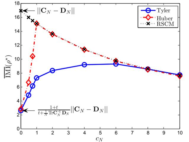
Fig. 4: Infinitesimal measure of influence vs. the aspect ratio  $c_N$ . The IMI is computed at the optimal regularization parameter (assuming clean data) that minimizes the quadratic loss of the estimator. Arrows indicate the IMI in the non-regularized case ( $\rho = 0$ ).  $[\mathbf{C}_N]_{ij} = .9^{|i-j|}$  and  $[\mathbf{D}_N]_{ij} = .2^{|i-j|}$ .
