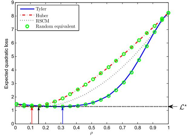
Fig. 1: Expected quadratic loss of different estimators as  $\rho$  varies, for  $N = 150$ ,  $n = 100$  ( $c_N = 3/2$ ), and  $[\mathbf{C}_N]_{ij} = .9^{|i-j|}$ , averaged over 100 realizations. Arrows indicate the estimated optimal regularization parameters for the considered estimators, while  $\mathcal{L}^*$  indicates the asymptotic, minimal quadratic loss.
