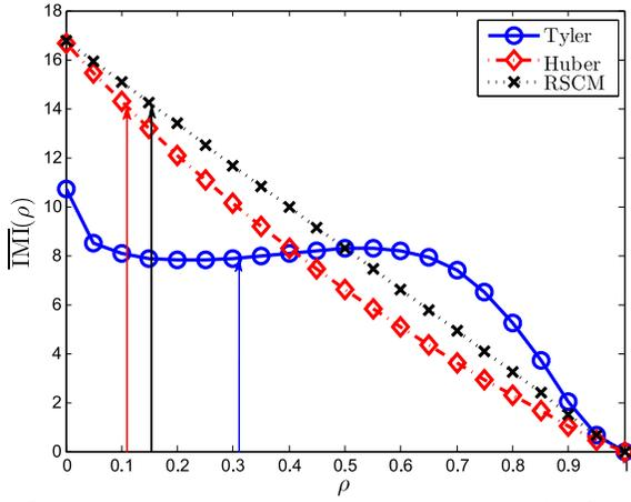
Fig. 5: Infinitesimal measure of influence for  $\rho \in (0, 1]$  ( $c_N = 3/2$ ). Arrows indicate the (oracle) optimal shrinkage parameter of the considered estimators in the absence of outliers.  $[\mathbf{C}_N]_{ij} = .9^{|i-j|}$  and  $[\mathbf{D}_N]_{ij} = .2^{|i-j|}$ .
