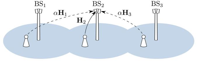
Fig. 1: Three cell example: BS<sub>2</sub> decodes the  $n$  streams from the UT in its own cell while treating the other signals as interference.
