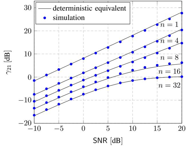
Fig. 3: SINR  $\gamma_{21}$  at the output of the MMSE receiver for different numbers of transmit signatures  $n$ ,  $N = 32$ ,  $\mathbf{P} = \frac{1}{n}\mathbf{I}_n$ ,  $L = 8$  and  $\alpha = 0.5$ .
