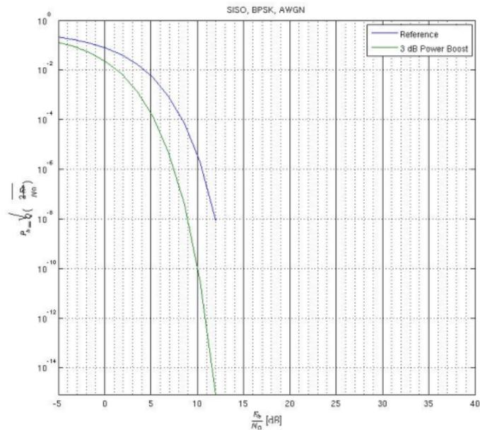
Figure: BER vs. SNR, BPSK, AWGN
