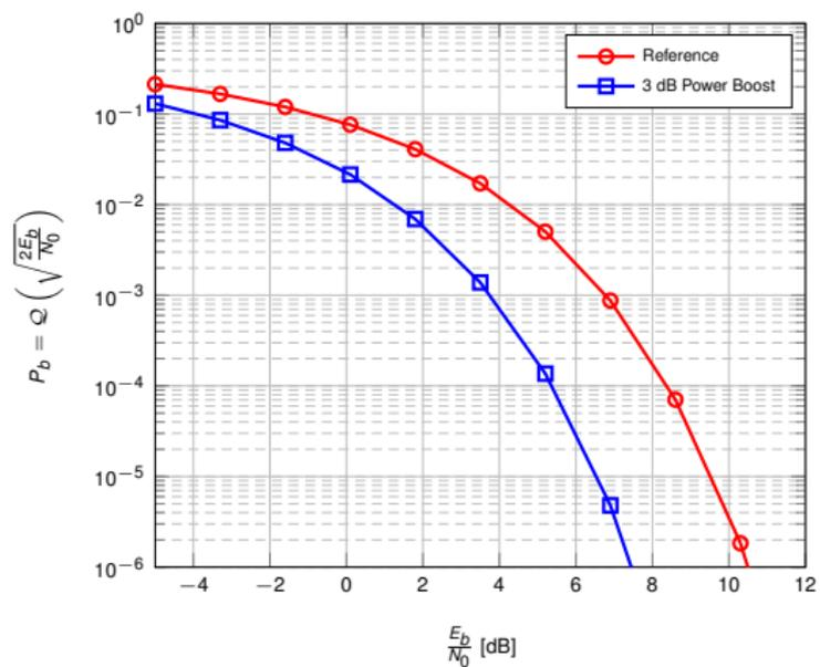
Figure: BER vs. SNR, BPSK, AWGN
